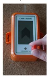
Hold a magnet to the right of the LED hole, approximately 10mm to the right of the LED, until the LED illuminates continuously. When this happens, move the magnet away from the Chevron and wait until the LED starts to flash . Once more, hold the magnet in the above position until the LED illuminates continuously. Now take the magnet away again. The website www.monitair.co.uk has a useful video showing how this is done.
